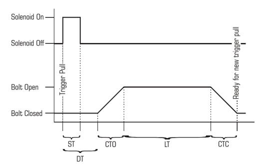
It's important to understand that ST and DT both start at the trigger pull, and that CTO will start after ST *or* DT is finished, whichever is the highest value of those two. Thus only the highest of those two count in the complete cycle time and the calculation of BPS. Needles to say it will almost never make sense to have ST higher than DT.
