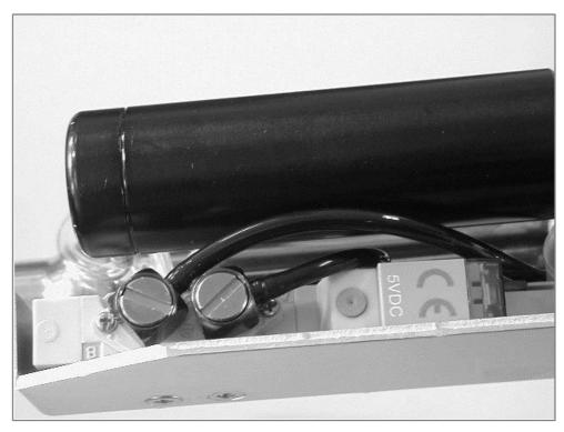
Swivel the fittings as needed, cut the hose-ends to final length and press them onto the front regulator and RAM.
