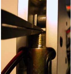
Then tighten the solenoid lock screw (don't overdo it - just snug it up and then a slight nudge) making sure nothing moves around. Remove the tool from behind the solenoid pin and notice that you now have a small gap between the solenoid pin and the sear actuator (tilt the frame a bit forward to let the solenoid pin drop back).
