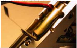
Put the tool behind the solenoid pin.
