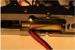
If there is not enough room for the spacer you have to shave a little material of the solenoid itself - do this very carefully (we are talking about 1/10 (0,1 millimeter) of a millimeter) using a small file or a Dremel with the appropriate tool.
