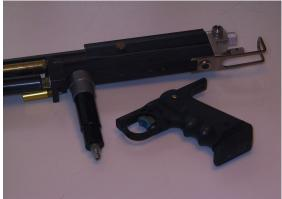
2. Remove the old 3-way valve by either cutting the three 1/8-inch hoses, leading to and from it, directly above the 3-ways fittings, or by disassembling the fittings. The latter may not be possible on some markers.
