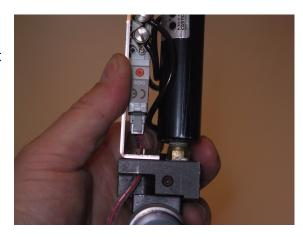
Put on some grip panels (not included) - the Racegun grip is compatible with all standard .45 frame grip panels. Plug in the battery before putting on the grip panels. Charge your grip for 4 hours and you are ready to "RACE"!
