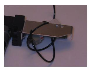
12. Note that the spacers go between the 5-way valve and the bracket.
