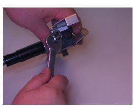
7. Screw the 3 supplied air fittings into the new 5-way valve.
