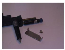
5. Install the bracket using the supplied hollow nut.
