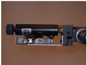
16. The sear lug screw should be set approx. 1-1.5mm (0,04-0,06") up measured from the bottom of the body as a starting point.
