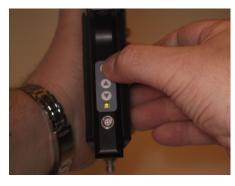
To turn the grip ON press the top button for 1 second—the led will light up green and the grip will beep once. To turn the grip OFF press the top button for 1 second, the grip will beep 3 times and the green led will turn off. Disconnect the battery if you are not going to use your grip for a longer period of time.
