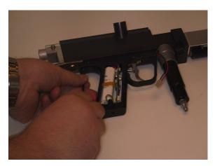
19. A wire wrap is included with your kit, thread one end on and twist it, to wrap it on the rest of the way.
