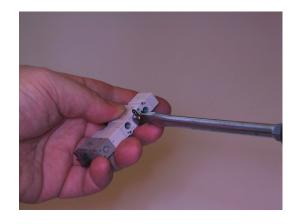
8. Valve side with 3 ports: fit 1 air fitting into the center port.
