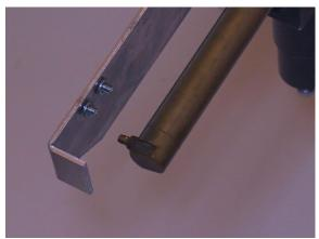
13. Take care not to over tighten the screws, the threads are very small and it's only aluminum.
