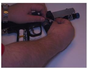
20. You need to connect the black and red lead to the 5-way valve. Put the connector through the hollow nut.
