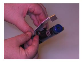
6. Use the 5/8" or 16mm wrench to tighten the bracket's hollow nut.
