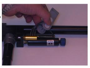
3. Unscrew the 5-way from the front block and remove it together with the trigger/actuating rod. It might be necessary to remove the LPR regulator first. If so, leave the LPR off.
