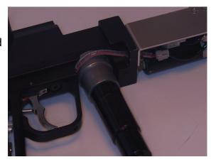
21. Connect the plug to the 5-way valve, it takes a little finesse to plug it in. The connector can only go in one way.
